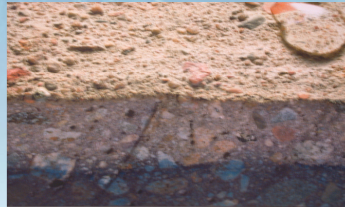
Penetration of Zycosil into Concrete
