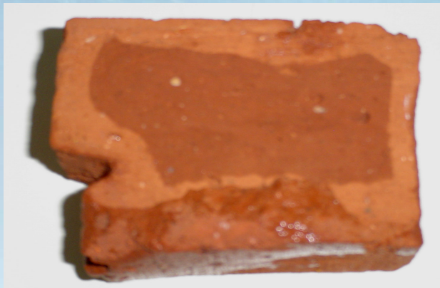
Penetration of Zycosil into brick
